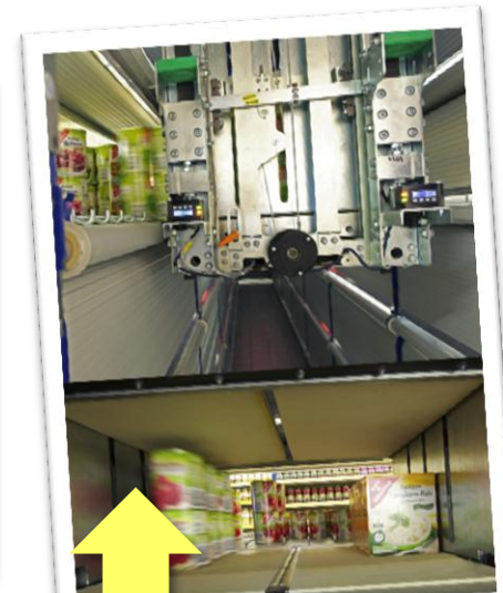
A horizontally and vertically moving shuttle carries out the replenishment.
