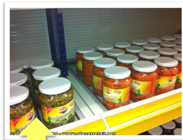
The shuttle and the shelf are divided by blinds which go up when items are replenished from behind.
